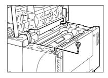
5 Close the drum cartridge cover and slide the platen unit to the original position.
